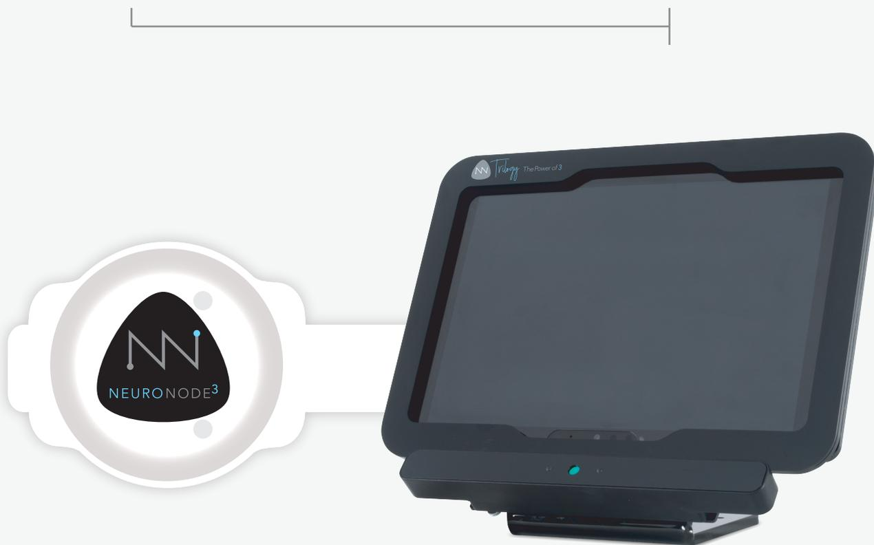
A non-adhesive, reusable electrode snaps to the bottom of the NeuroNode<sup>3</sup> which then snaps into the NeuroBand. The NeuroBand is a customizable comfortable band which anchors the NeuroNode<sup>3</sup> directly to the chosen muscle site.
